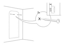
(3.) Place the hangers at the back of the mirror over the screws.
