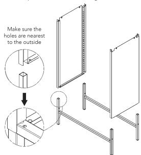
3. Assemble the back panels (B) onto the standing structure and bend the tabs in the four corners, to fix in place
