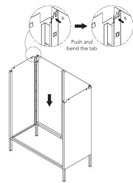
Assemble the back panels (B) by slotting them together.
