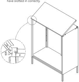
7. Insert the metal post (H) and washer (I) in the hole in the leg. Hinge the door (C) onto the post. Push down and hold the metal hinge button at the top of the door. Slide the door in place, releasing the hinge to fix into position within the top panel. Repeat for second door.
