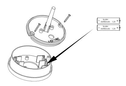
Once fitted with a new battery, charge the solar panel in sunlight to activate it the light
