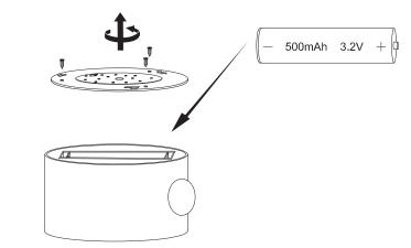
Once fitted with a new battery, charge the solar panel in sunlight to activate it the light
