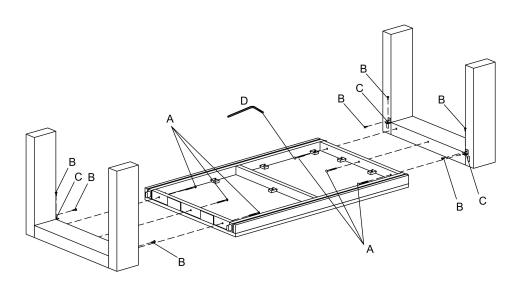
FIX THE LEGS WITH THE TOP USING A & B SCREWS
