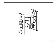
Tighten the strap until snug and cut off the end.
