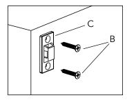
Mark and drill holes for screws, installing one anti-tip bracket onto the back of your furniture piece in a vertical position.
