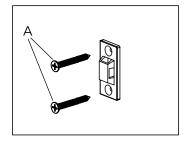
Mark and drill holes for screws before installing another bracket onto the wall, taking care to line it up with the mounted furniture bracket.
