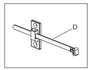
Thread the strap through both anti-tip brackets mounted onto the wall and your furniture.
