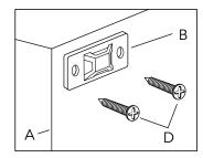
Mark and drill holes for screws, installing one anti-tip bracket onto the back of your furniture piece in a horizontal position.
